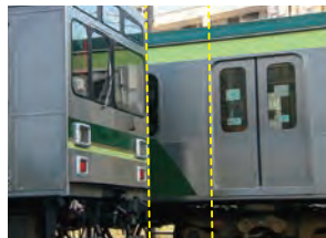
No Rolling Shutter Artifacts with Global Shutter
