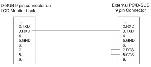
Do not connect anything to pins 1, 4, 6, 7, 8, or 9 on the monitor side (or else, a malfunction of the monitor may occur).
