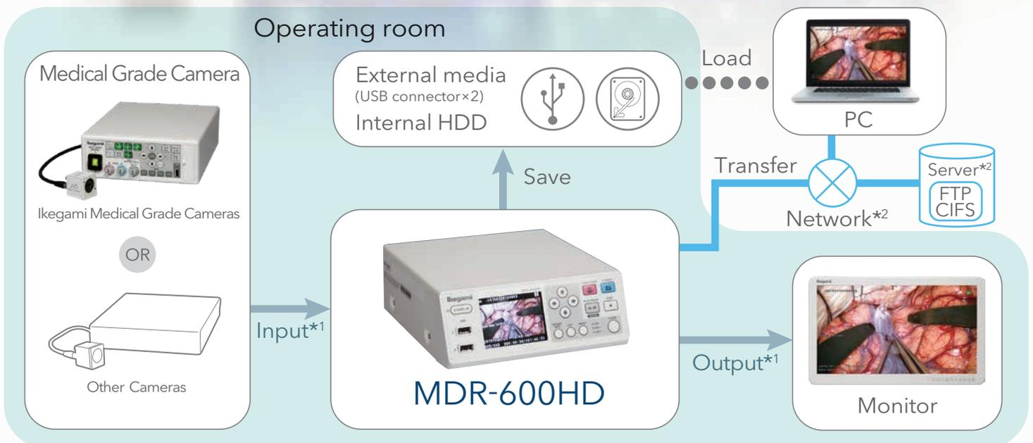
\*1 Digital:SD-SDI/HD-HDI/DVI-D Analog:COMPOSITE/S-VIDEO.Input signal and output signal must be same.
